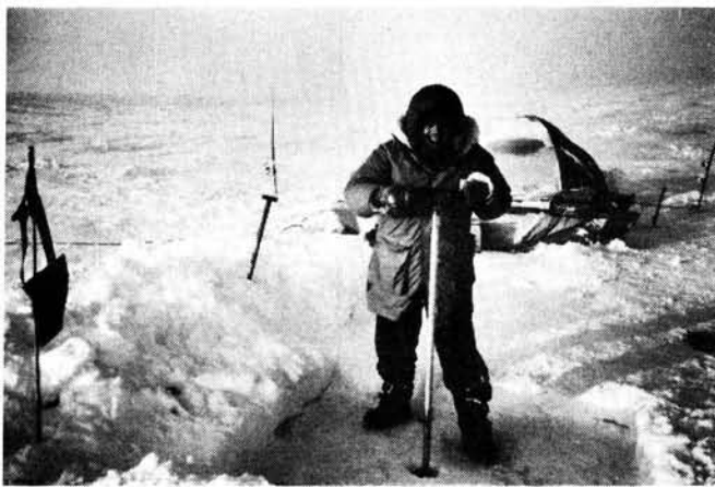
Hand-drilling ice-cores to 10m takes two days at -45^{\circ}\text{C} , east of Ward Hunt Island
